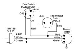
Figure 18 - Wiring Diagram For Blower Accessory Standard Installation
